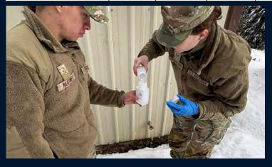
A1C Ramanouskaya and A1C Martinez from the 92nd Bioenvironmental Engineering flight performing water sampling at a Geographically Separated Unit (GSU). Samples are taken and then transported to Anatek laboratory for analysis.
